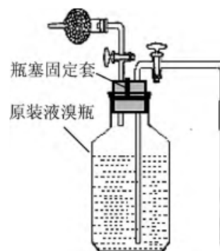
Fig 2 Device for transferring liquid bromine safely
